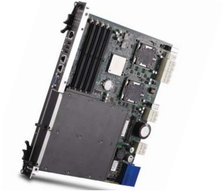
Figure 1 Adlink's aTCA-6900 features two quad-core Intel Xeon processors and dual mezzanine-card bays to extend the performance of high-availability AdvancedTCA systems.
