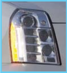
Figure 1 The Cadillac Escalade Platinum is one of the first production cars to use HB LEDs for headlights. LEDs also find use as indicators, taillights, and cabin lights.
