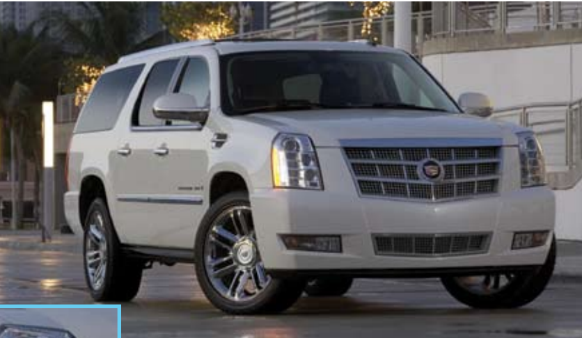
Figure 1 The Cadillac Escalade Platinum is one of the first production cars to use HB LEDs for headlights. LEDs also find use as indicators, taillights, and cabin lights.
