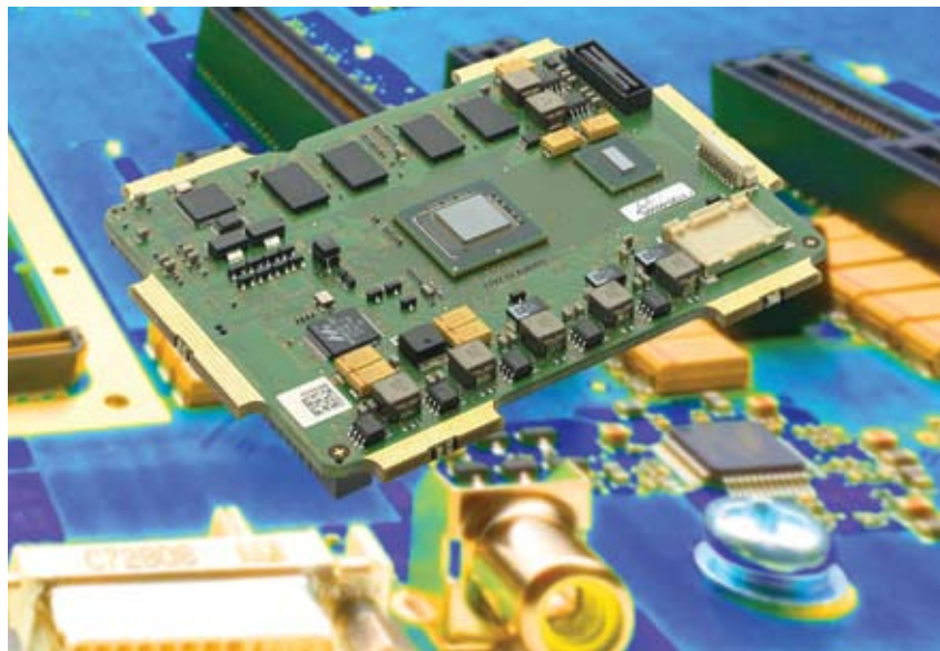
Figure 2 The XM1 computer module targets harsh-environment applications by integrating advanced cooling technologies, the latest serial buses, and rugged components.
