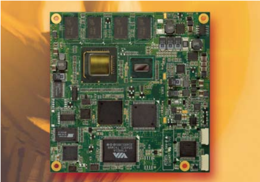
Figure 3 With low-power- and portable-system applications in mind, Congatec recently announced the high-performance conga-CA processor module in a standard COM Express form factor.
