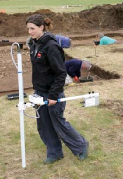
Figure 2 This field researcher is using a Grad601 flux-gate gradiometer at an archeological-dig site (courtesy Bartington).
