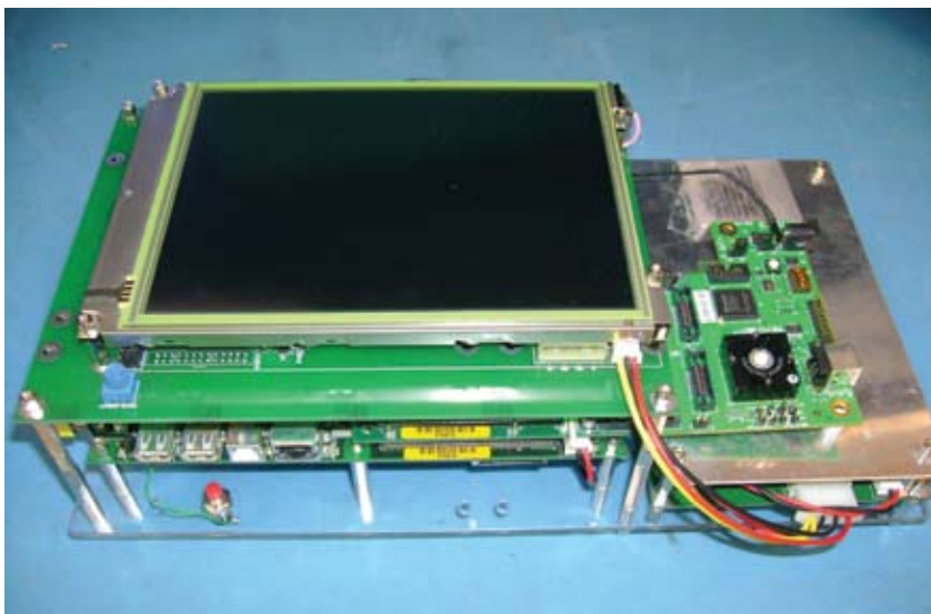
Figure 1 Synopsys designers created a SystemC transaction-level model of this development board to enable hardware/driver co-design.
