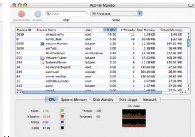
(a) (b) Figure 5 The virtual-machine manager consumes perceptible CPU resources in both single-core (a) and dual-core (b) virtualization configurations, even with the virtualized OS at idle.
