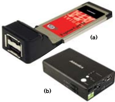
Figure 2 Addonics Technologies' ExpressCard eSATA adapter (a) and portable dual-drive RAID enclosure (b) were among the key pieces of hardware I employed.
