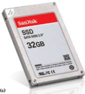
Figure 4 I used two of Intel's multilevel-cell flash-memory-based solid-state drives (a), which enabled me to do some interesting RAID 0 testing. I also tested a single-level-cell solid-state drive from Samsung (b) and an older design from Sandisk (c).
