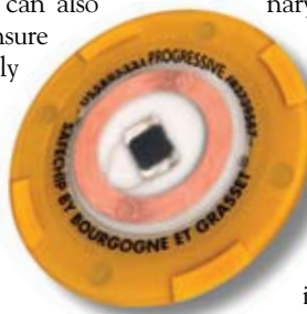
Figure 4 The Safechip from Gaming Partners International works in casino-chip-tracking and security applications and features a 256-bit transponder IC by NXP Semiconductors.
