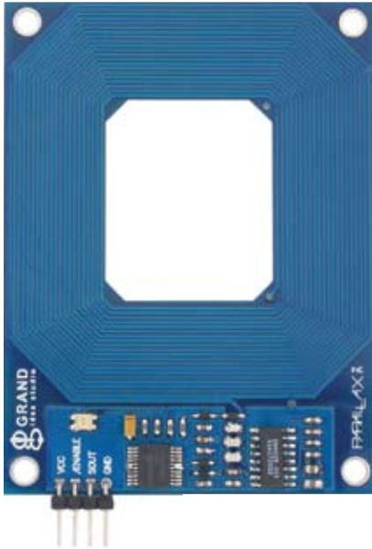
Figure 2 Selling for less than $40, the Parallax reader provides a low-cost, entry-level device to read passive-RFID tags for experimentation or embedded-system applications.
