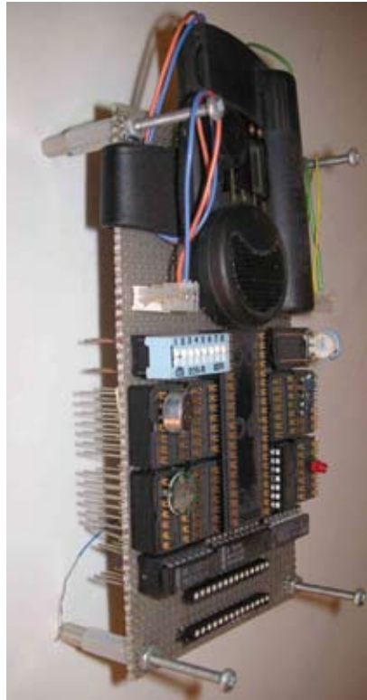
Figure 3 Because of low operating frequencies, wire-wrap techniques work well in this toy-watch-recorder prototype.
