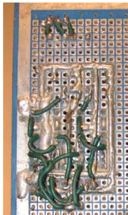
Figure 2 Soldering discrete wires to parts on a perforated board is an acceptable way of prototyping circuits.
