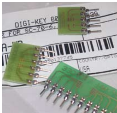
Figure 1 A huge selection of adapter boards spread out tiny packages to 100-mil spacing.
