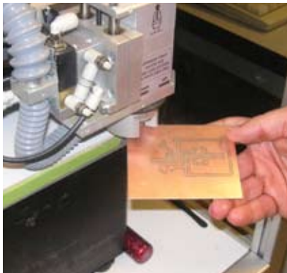
Figure 4 This LPKF mill can route out prototype boards in less than an hour (courtesy National Semiconductor).
