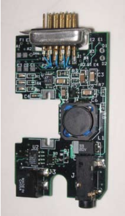
Figure 5 Only a board house can make small boards with fine trace widths and spacings.
