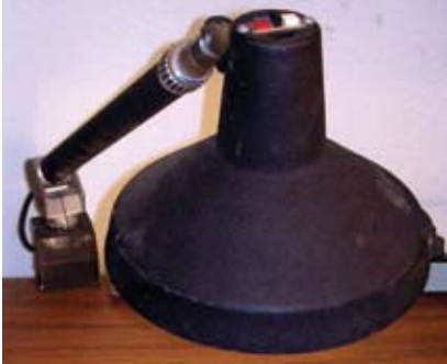
Figure A Articulated lamps with fans or magnifiers are essential to get light where you need it.
