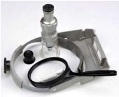
Figure C This selection of magnifiers includes an eye loupe, a headband with magnifying lenses, and a handheld microscope.
