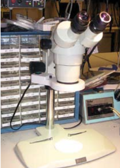
Figure E This Motic microscope comes with a ring illuminator that uses a compact fluorescent bulb. Newer ring illuminators use LEDs (courtesy National Semiconductor).
