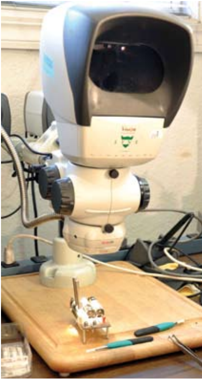
Figure F This Lynx model Dynascope from Vision Engineering provides a stereo image by use of a lenticular rotating mirror.
