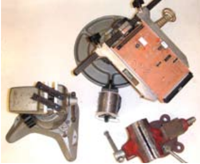
Figure H Panavise makes conventional vises as well as those meant to hold boards while you solder in components. A cheap iron vise also comes in handy for mechanical work.
