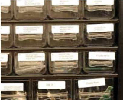
Figure 1 It is a good idea to arrange all the parts for a board in a cabinet just for that purpose. It makes assembly, repair, and reordering much easier.
