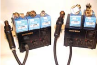
Figure J Hakko hot-air soldering guns are useful for soldering or remove surface-mount parts. You can use the second unit to heat large copper planes from underneath.
