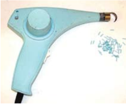
Figure K A small heat gun is more useful than larger, heavier units for shrink tubing and spot-heat components.
