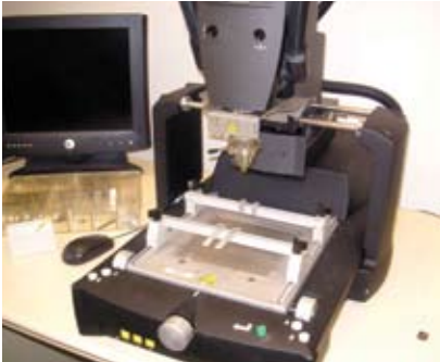
Figure M An OK International hot-air rework station has a dual-view camera that can slide out to help align the component you are soldering onto your board (courtesy National Semiconductor).
