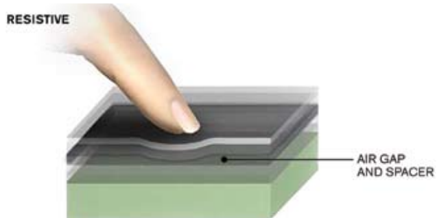
Figure 1 With resistive touchscreen technology, when you apply pressure to the outer layer, it makes contact with the inner layer, leading to an electrical contact.
