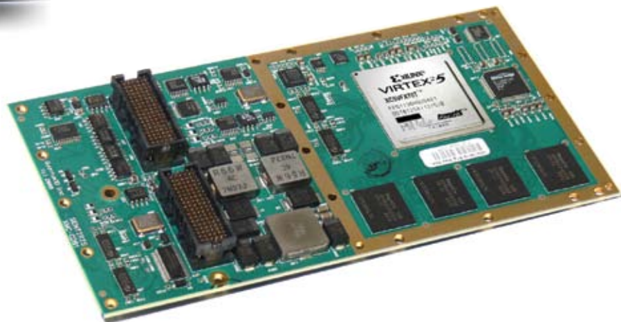
Figure 3 The Sentiris AV1 PCI express mezzanine card from Quantum3D fights obsolescence by incorporating an FPGA-based video- and graphics-processing core.
