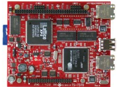
Figure 5 TS-7370 from Technologic Systems includes a user-programmable FPGA allowing you to create a custom interface to most color TFT-LCD panels.
