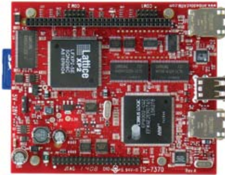
Figure 5 TS-7370 from Technologic Systems includes a user-programmable FPGA allowing you to create a custom interface to most color TFT-LCD panels.
