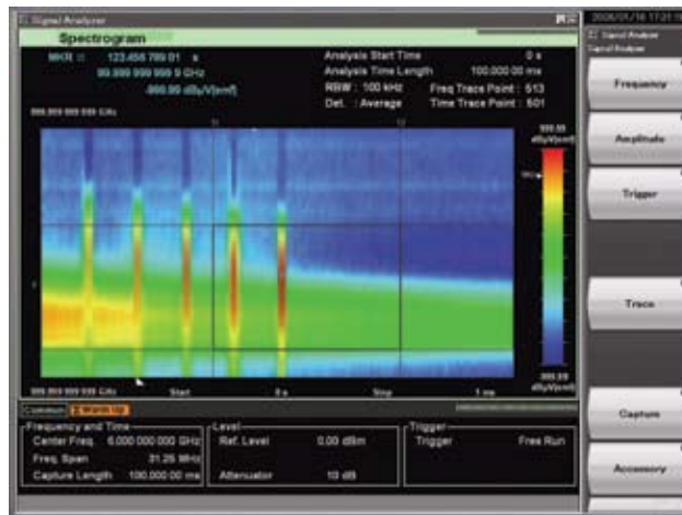
Figure 3 A signal analyzer's spectrogram function shows a 3-D representation of an LTE signal. Vertical cursors allow users to select a particular slice of data in the time domain, and horizontal cursors allow users to designate a frequency of interest (courtesy Anritsu).
