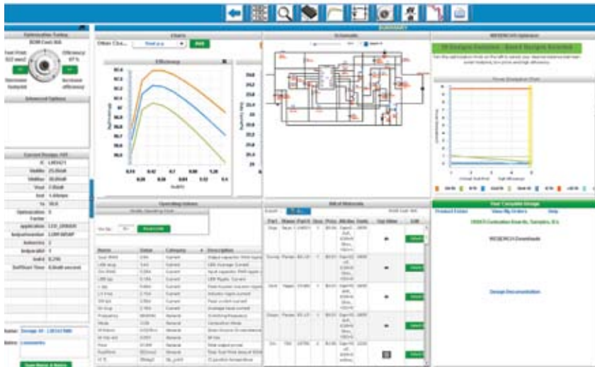
Figure 3 Webench has an LED-driver-design function with a powerful interface (courtesy National Semiconductor).
