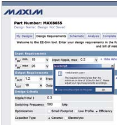
Figure 6 Maxim's EE-Sim provides a dialog box to warn you that the circuit will not work unless you change the specifications or the part.
