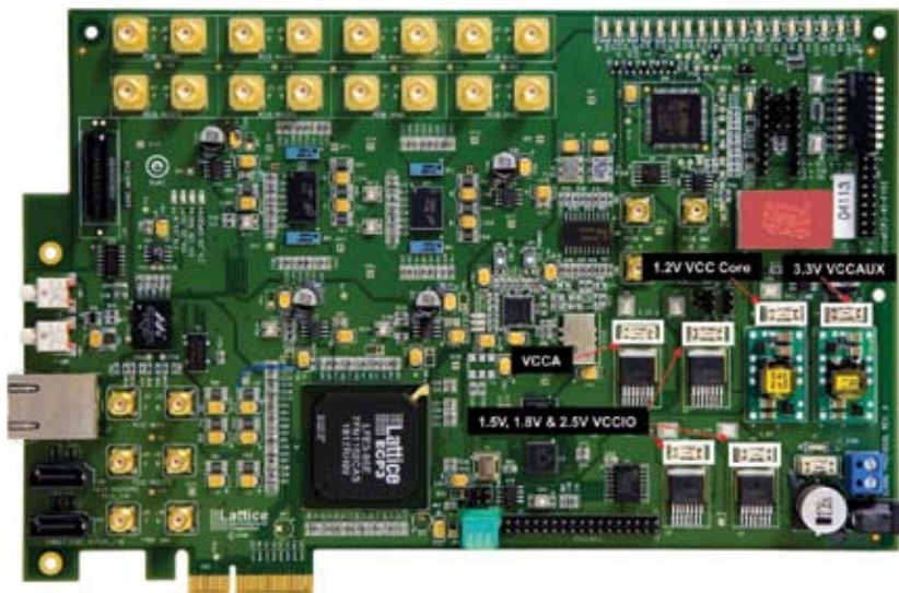
Figure 2 Development boards, like this one from Lattice Semiconductor, often provide low-impedance access points for monitoring current on the FPGA's supply rails.
