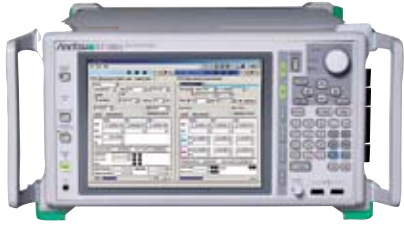
Figure C I/O cards for Anritsu's MP1800A signal analyzer let you modulate and analyze 40- and 100-Gbps optical signals.
