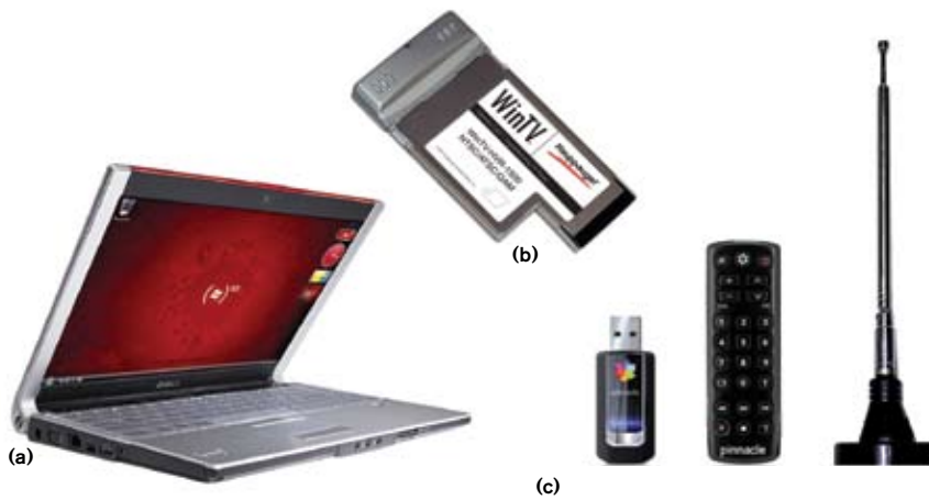
Figure 5 A Dell XPS M1330 laptop (a) became my digital PVR in conjunction with the Media Center application that comes with Windows Vista Ultimate and a Hewlett-Packard-branded version of Hauppauge's HVR-1500 ExpressCard TV tuner (b). I also tried Pinnacle's USB-based PCTV HD mini stick (c), but it created artifact-filled recordings, counterbalancing the unit's robust software suite and integrated "signal booster."
