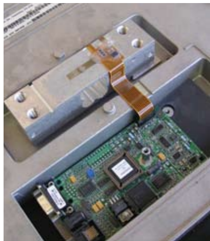
Figure 2 This Mettler Toledo scale has a precision load cell with a memory chip for linearization and calibration.
