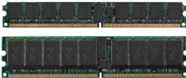
Figure 6 The very-low-profile DIMMs are essentially the same as the standard DIMMs but at 60% of the height.
