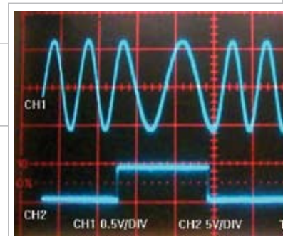
Figure 2 The FSK modulator's output changes frequency based on a digital input.
