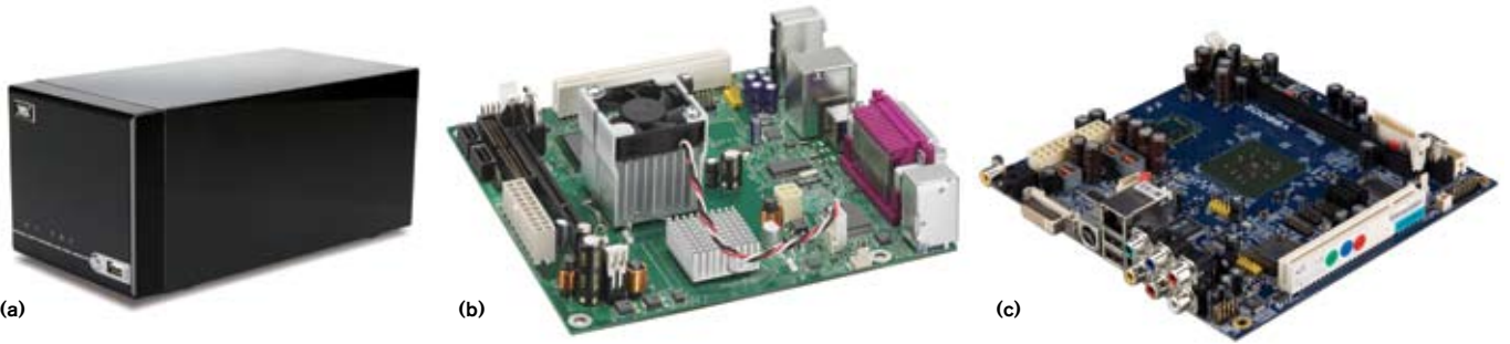
Figure A Via's Artigo A2000 NAS-tailored design embeds a 1.5-GHz CPU and a nearly silent system fan (a), whereas Intel's single- and dual-core Atom boards support a more modern CPU architecture (b). For stringent performance demands, consider Via's VB8002 board, which the company based on its most recent Nano CPU, complete with a three-way-superscalar, out-of-order architecture (c).
