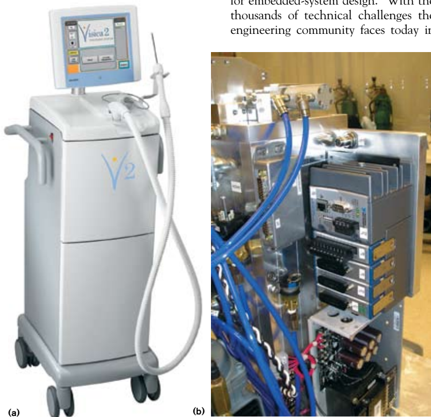
Figure 1 The Visica 2 cryoablation system for the treatment of tumors (a) went from a requirements document to first revenue in 14 months, according to system engineer Jeff Stevens (courtesy Sanarus). Stevens used LabView to develop code for the CompactRIO platform (b) that served as the embedded engine in Visica 2 (courtesy National Instruments).
