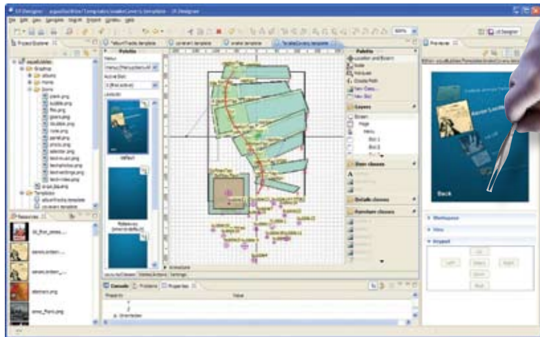
Figure 4 Domain experts—in this case, creative and usability specialists—can now contribute directly to the development of embedded products’ user interfaces by employing the drag-and-drop Nucleus Graphics Designer tool (courtesy Mentor Graphics).
