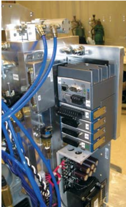
Figure 1 The Visica 2 cryoablation system for the treatment of tumors (a) went from a requirements document to first revenue in 14 months, according to system engineer Jeff Stevens (courtesy Sanarus). Stevens used LabView to develop code for the CompactRIO platform (b) that served as the embedded engine in Visica 2 (courtesy National Instruments).
