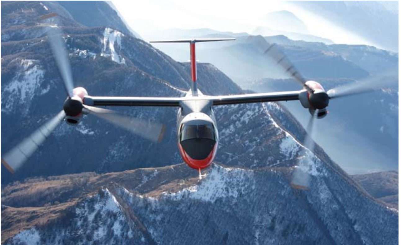
Figure 3 One of two BA609 tilt-rotor aircraft undergoes flight testing, flying in airplane mode over the Alps in northern Italy (courtesy Bell/Agusta Aerospace Co).
