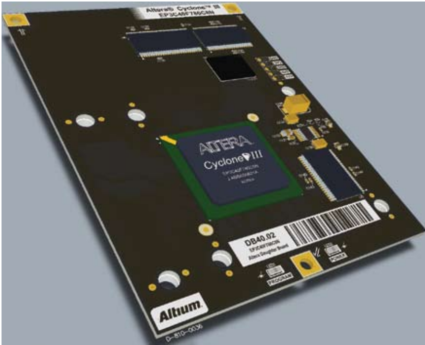
Figure 6 In conjunction with the Altium Designer unified-electronics-design tool, this daughterboard for its desktop NanoBoard reconfigurable-hardware-development platform targets Altera's Cyclone III EP3C40 FPGA in a 780-bump BGA package (courtesy Altium).
