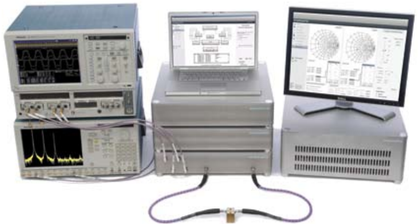
Figure 4 Tektronix teamed up with Mesuro at IMS 2009 to demonstrate open-loop, active-harmonic, load-pull-system measurements using the Tektronix arbitrary-waveform generator and sampling oscilloscope plus the Mesuro MB 20 system.
