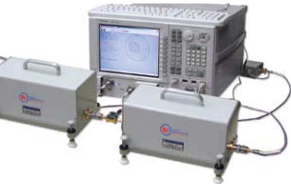
Figure 3 In conjunction with Maury Microwave, Agilent at IMS 2009 demonstrated the measurement and simulation of nonlinear component behavior, using an Agilent PNA-X nonlinear-vector-network analyzer and Maury Microwave tuners and software (courtesy Agilent Technologies).
