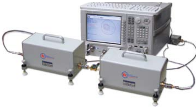
Figure 3 In conjunction with Maury Microwave, Agilent at IMS 2009 demonstrated the measurement and simulation of nonlinear component behavior, using an Agilent PNA-X nonlinear-vector-network analyzer and Maury Microwave tuners and software (courtesy Agilent Technologies).
