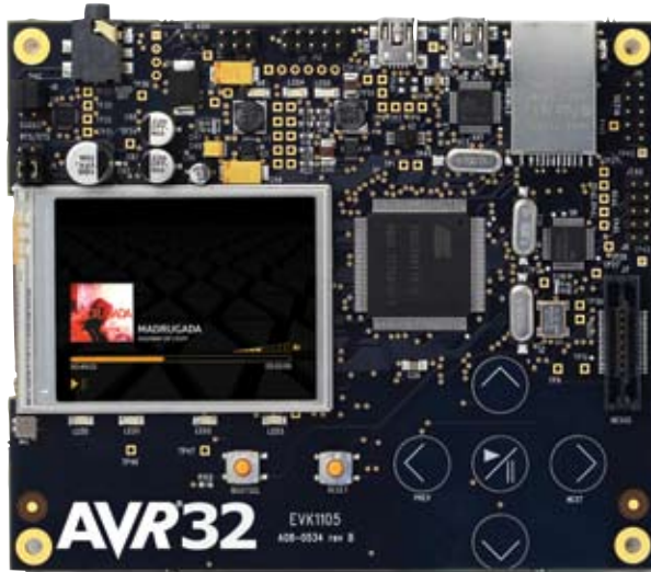
Figure 2 The ATEVK1105 evaluation kit supported the port to Atmel's AVR32 processor.
