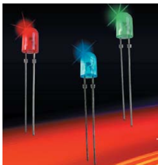
LEDs are moving up the intensity scale for outdoor-signage uses, as the OVL series demonstrates. The devices are available in a range of colors and 3-, 4-, and 5-mm sizes.
