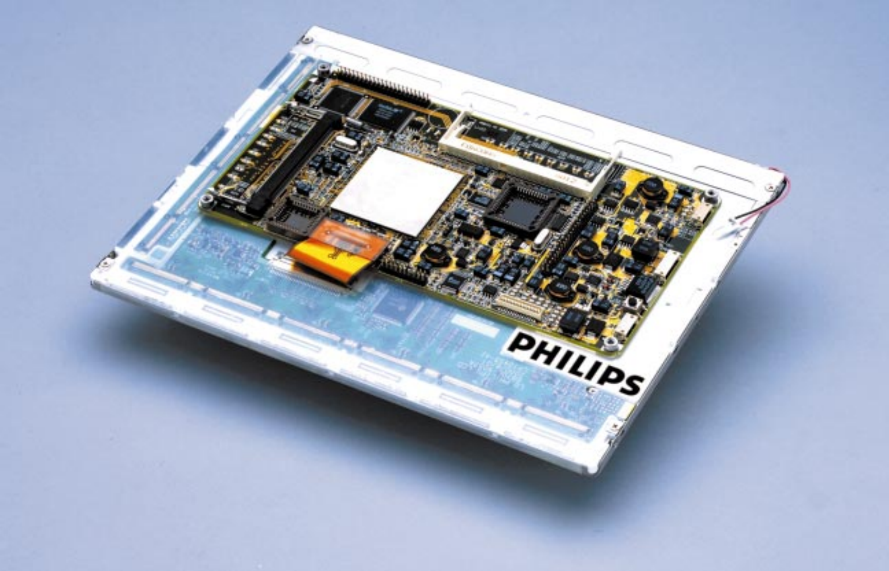
Philips' Net Display Module integrates Web-appliance electronics within an LCD panel.
