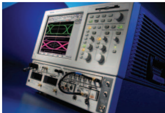
The modular TDS8200 sequential equivalent-time sampling oscilloscope and 82A04 phase-reference module allow bandwidths as great as 70 GHz, incorporate a single-ended and differential clock-recovery system, and exhibit less-than-200-fsec-rms jitter.
