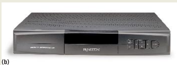
A rooftop antenna on a 20-foot pole (a) and a DTV receiver (b) enable your progressive-scan monitor to display terrestrial-digital-television broadcasts (courtesy Terk and Princeton Graphics, respectively).
