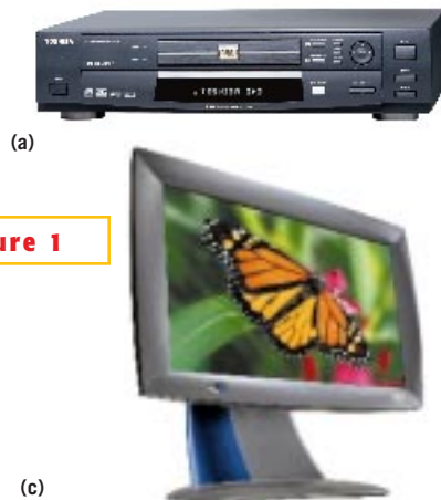
A progressive-scan DVD player (a) also acts as a high-quality video source for other deinterlacers for display on wide-screen CRT (b) and LCD (c) monitors (courtesy Toshiba, Princeton Graphics, and Silicon Graphics, respectively).
