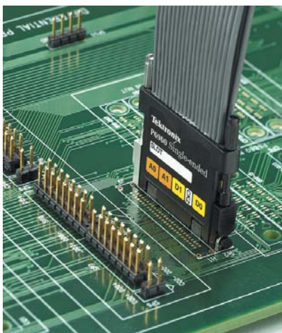
The latest probe design from Tektronix still offers 34 signal lines, but in a reduced footprint and with just 0.5-pF loading.
