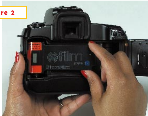
Silicon Film Technologies designed (e)film to drop into a 35-mm SLR camera.
