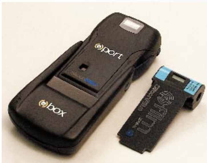
Figure 1 The EFS-1 system includes (e)film for image capture, (e)port for image transfer to a PC, and (e)box for temporary bulk-image storage (courtesy Silicon Film Technologies).
