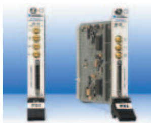
The mixed-signal test suite includes seven waveform-digitization, -generation, and -support modules in single-width PXI format.
