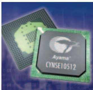
The Ayama 10000 NSE family of TCAM-based search engines provides as many as 266 million searches/sec.
