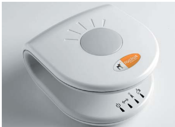
The Ruckus Wireless MF2900 video-capable 802.11g access point and router features a six-element smart antenna in the upper half of the clamshell and dynamic software control that forms signal beams through 63 antenna patterns.
