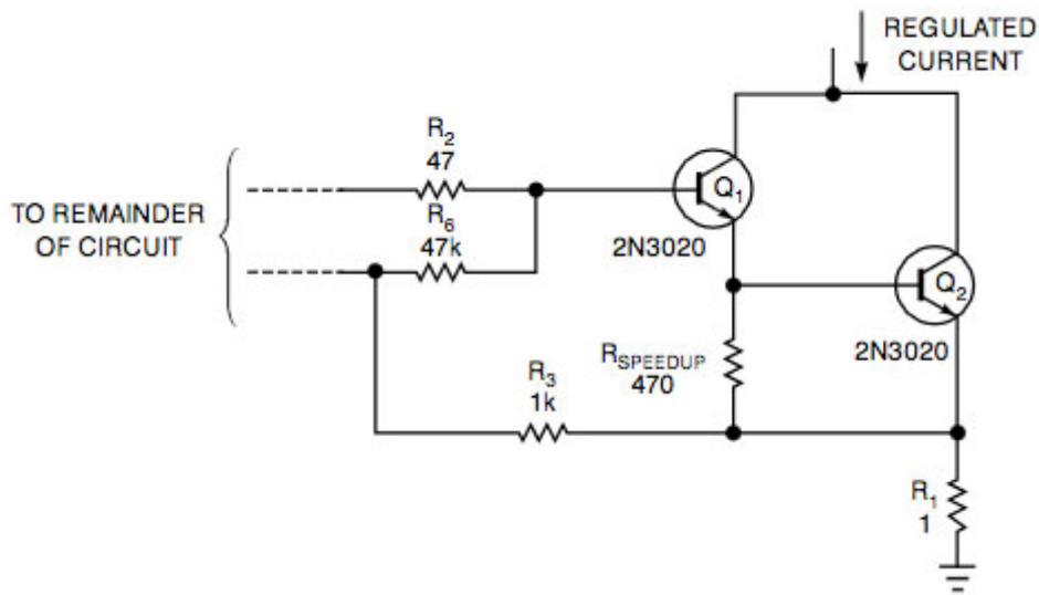
**Figure 4** Adding R<sub>SPEEDUP</sub> improves the performance of a two-transistor Darlington output stage.
