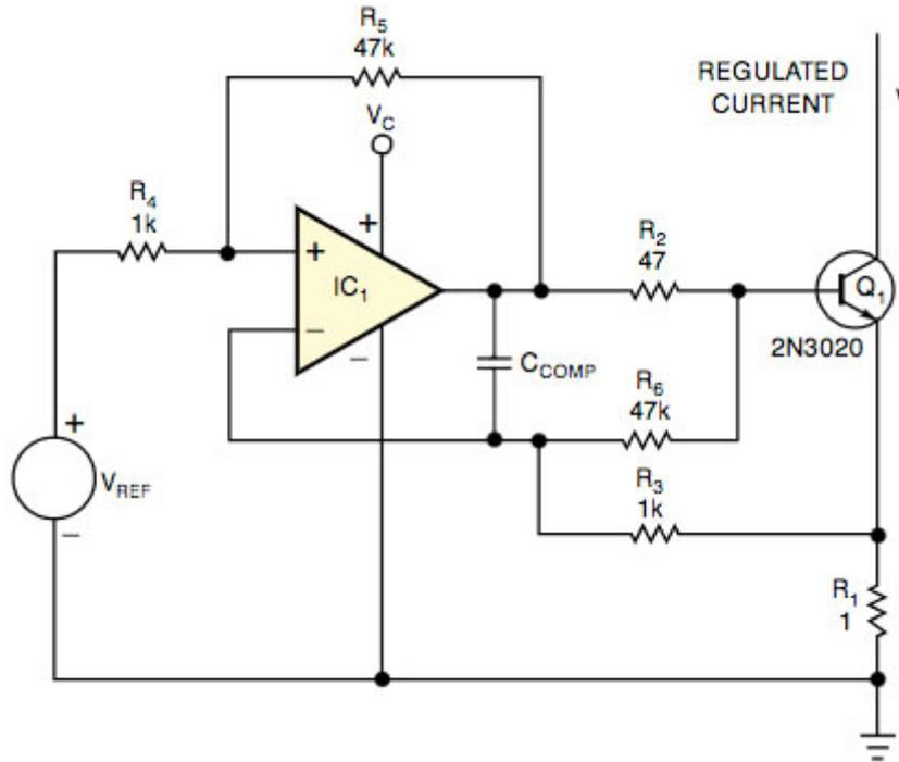
**Figure 3** You can further simplify the current sink's design by adding only two resistors,  $R_5$  and  $R_6$ , to the original in Figure 1. The output-current equation remains  $I_{OUT}=(V_{REF}/R_1)$ , as in Figure 2.
