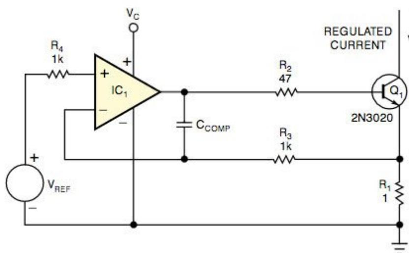
**Figure 1** This typical quickly responding constant-current sink uses a bipolar transistor but suffers from base-current-induced error. Its normal output current is  $I_{OUT}=(V_{REF}/R_1)-I_B$ .
